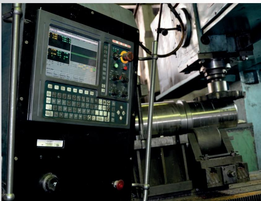
We use the special rolls grinding and milling machines with digital control for finishing.
